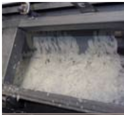
Formation of stable white Prifex® Flaked fats at the cooled drum.
